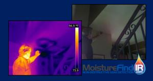
During our infrared investigation, SoCal Infrared Thermographers can instantly image entire rooms, inspecting places that can't be physically reached with moisture meters. This reveals wet conditions that can't be seen with the naked eye such as behind wallpaper, which doesn't readily water stain.
