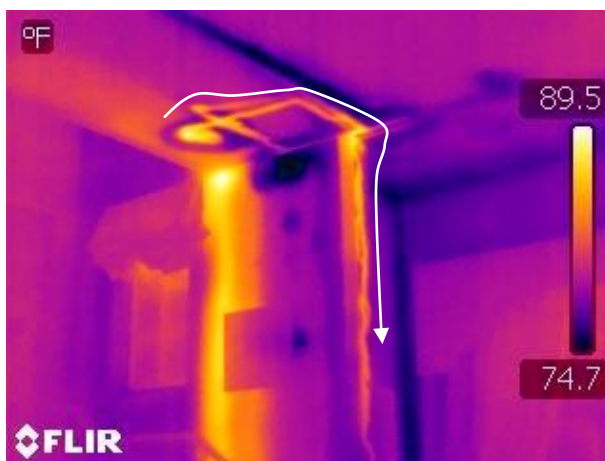
Water testing showing water travel
