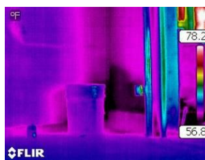
Thermal image showing wet area of wall
