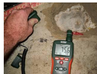
Portions of slab chipped away in areas of high moisture. Notice the Red pipe in slab (radiant heating)
