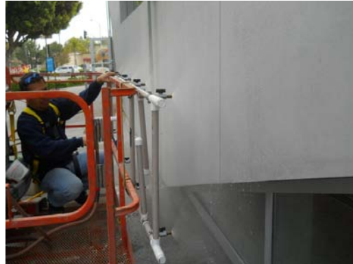
Figure 22. Leaks were found at three brand new buildings at this complex. The client had complained to builder of many leaks noted at windows.
