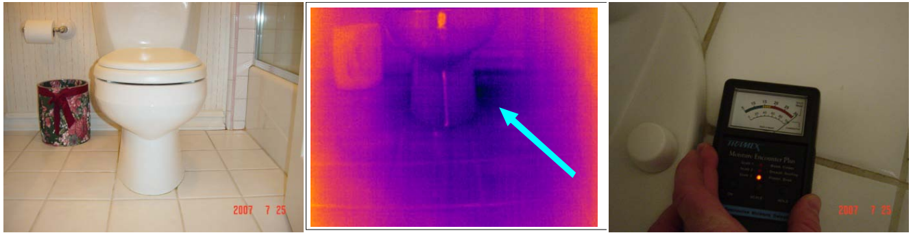
Figure 5. The room above the location of moisture damage was quickly viewed with a thermal camera and revealed a colder area at right side of toilet. When read with a moisture meter, this area was found to have 100% moisture. For comparison, the left side of toilet showed high as well, but the center of bathroom showed 0%. Thermal imaging helped to diagnose the leak's source: a failed wax seal and loose bolt on the toilet.
