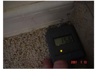
Figure 31. Client's complaint was that the shower leaked, but the shower had not been used in over a year. Thermal imaging in combination with the use of moisture meters confirmed elevated moisture at corner of wall (rather than close to shower as would be suspected).
