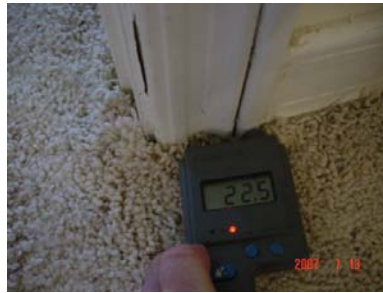
Figure 31. Client's complaint was that the shower leaked, but the shower had not been used in over a year. Thermal imaging in combination with the use of moisture meters confirmed elevated moisture at corner of wall (rather than close to shower as would be suspected).
