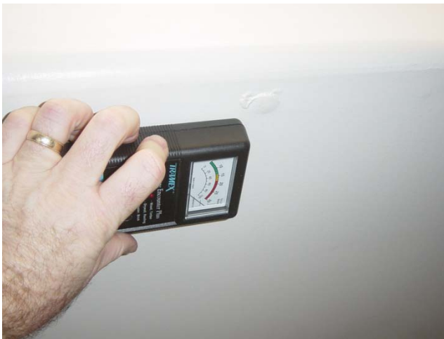
Figure 18. The wet area identified in thermal image was first confirmed with a moisture meter at 100% and then to the source. The roof had a steep slope with an upper roof cascading over, causing water to first hit the structure and bypass the counter flashing therefore leading to moisture entry. The suggested repair on this home involved a new design for a valley flashing versus the suggested roof replacement.
